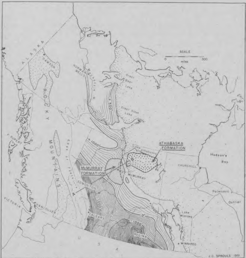
Fig. 1. Western Canada sedimentary basins showing (1) contours on the Paleozoic surface (datum—sea level), and (2) relationships of the McMurray formation. (Published by permission of Imperial Oil Limited, Calgary.)
