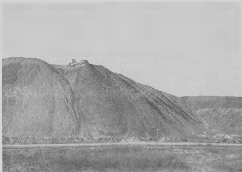
View of the overburden dump. Vertical height at this point is 150 ft. No difficulty has been experienced with slides except when depositing wet material on swampy ground covered with muskeg.
