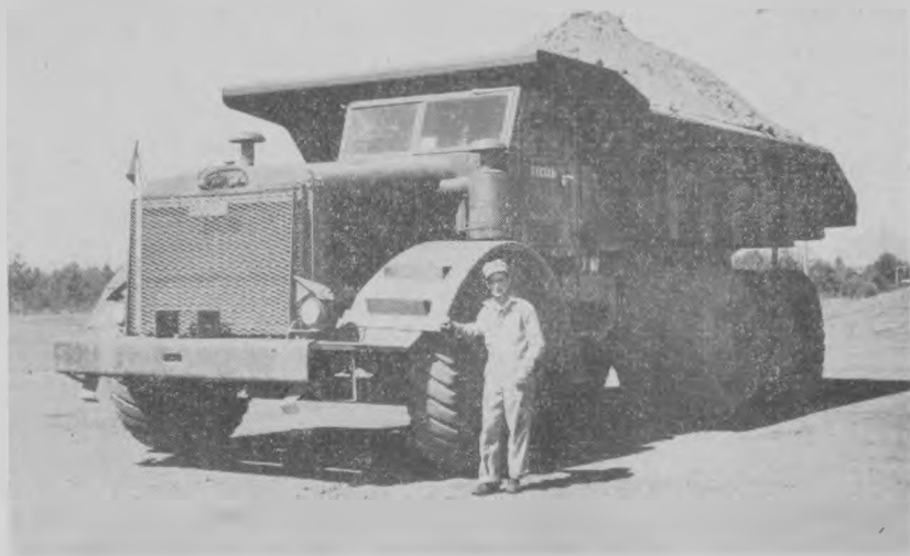
A 50-ton experimental model LLD Euclid truck having two 300-h.p. Cummins engines driving tandem rear axles. Note the thermostatically controlled shutter over the radiator core. The cooling fans are also controlled by the temperature of the engines. Capacity of the box is 32 cu. yd. water level.
