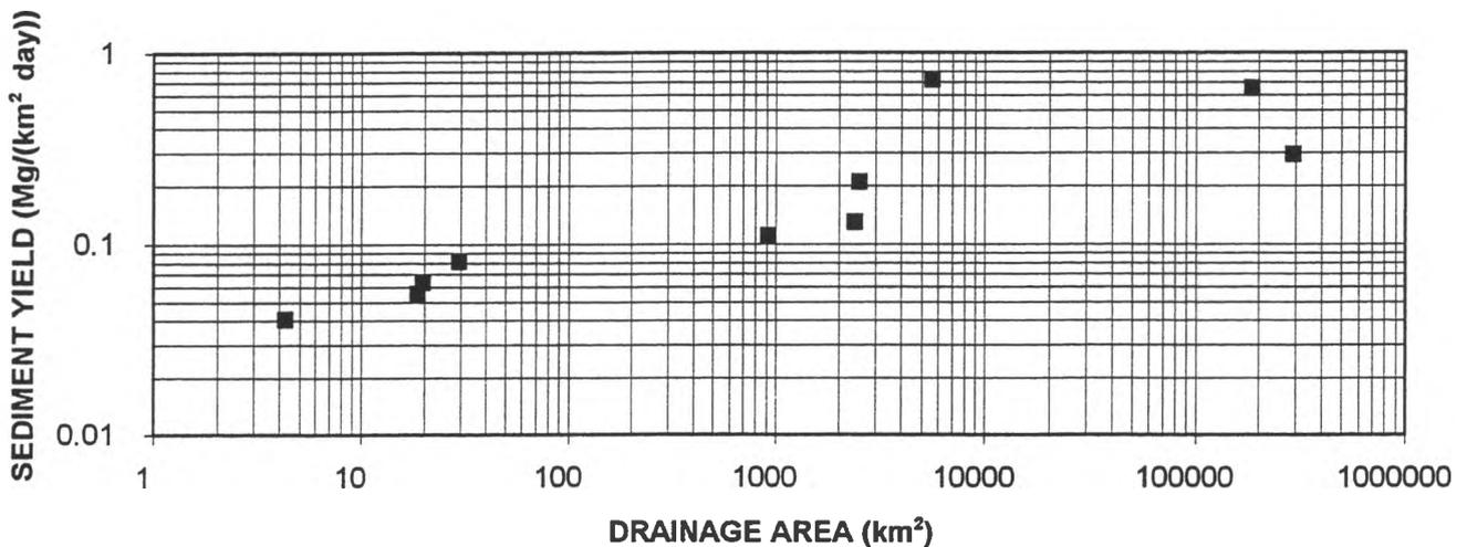
**Figure 2. The variation of specific sediment yield (sediment yield per unit area) with drainage area in the Peace River drainage basin. The data are based mainly on tributary streams and include no stations within the mountains.**
