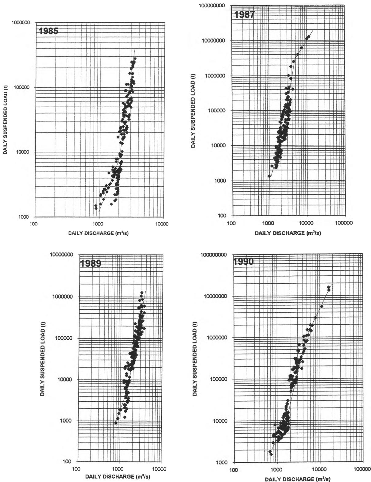
**Figure 10. Daily suspended load rating curves for various years post-regulation years, Peace River at Peace River. 1985 and 1989 were low flow years ( $Q_{\max} < 4000 \text{ m}^3 \text{ s}^{-1}$ ), whereas 1987 and 1990 were high flow years ( $Q_{\max} > 10\,000 \text{ m}^3 \text{ s}^{-1}$ ).**
