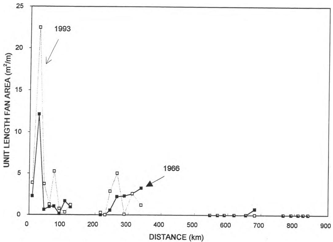
**Figure 24. Area of alluvial fans within the Peace River valley flat per unit length of channel, by subreach; distances downstream from the British Columbia - Alberta border.**
