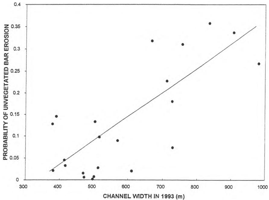
**Figure 28. Correlation of the probability of erosion of unvegetated bars between 1968 and 1993 with channel width in 1993 (subreach means).**
