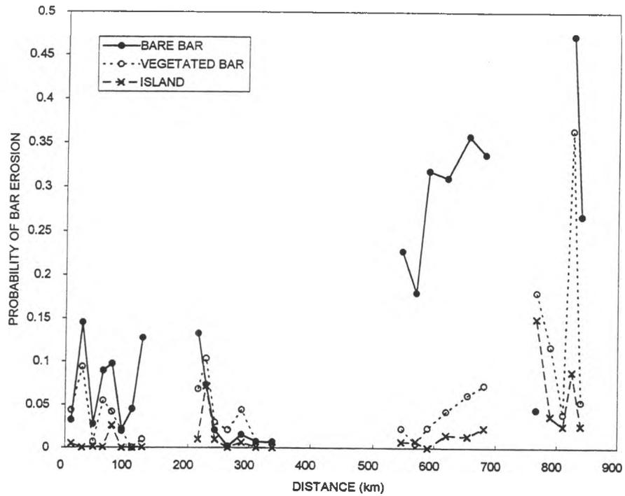
**Figure 27. Probability of erosion for bare bars, vegetated bars and islands between 1968 and 1993, by subreach means, along Peace River downstream from the British Columbia - Alberta border.**
