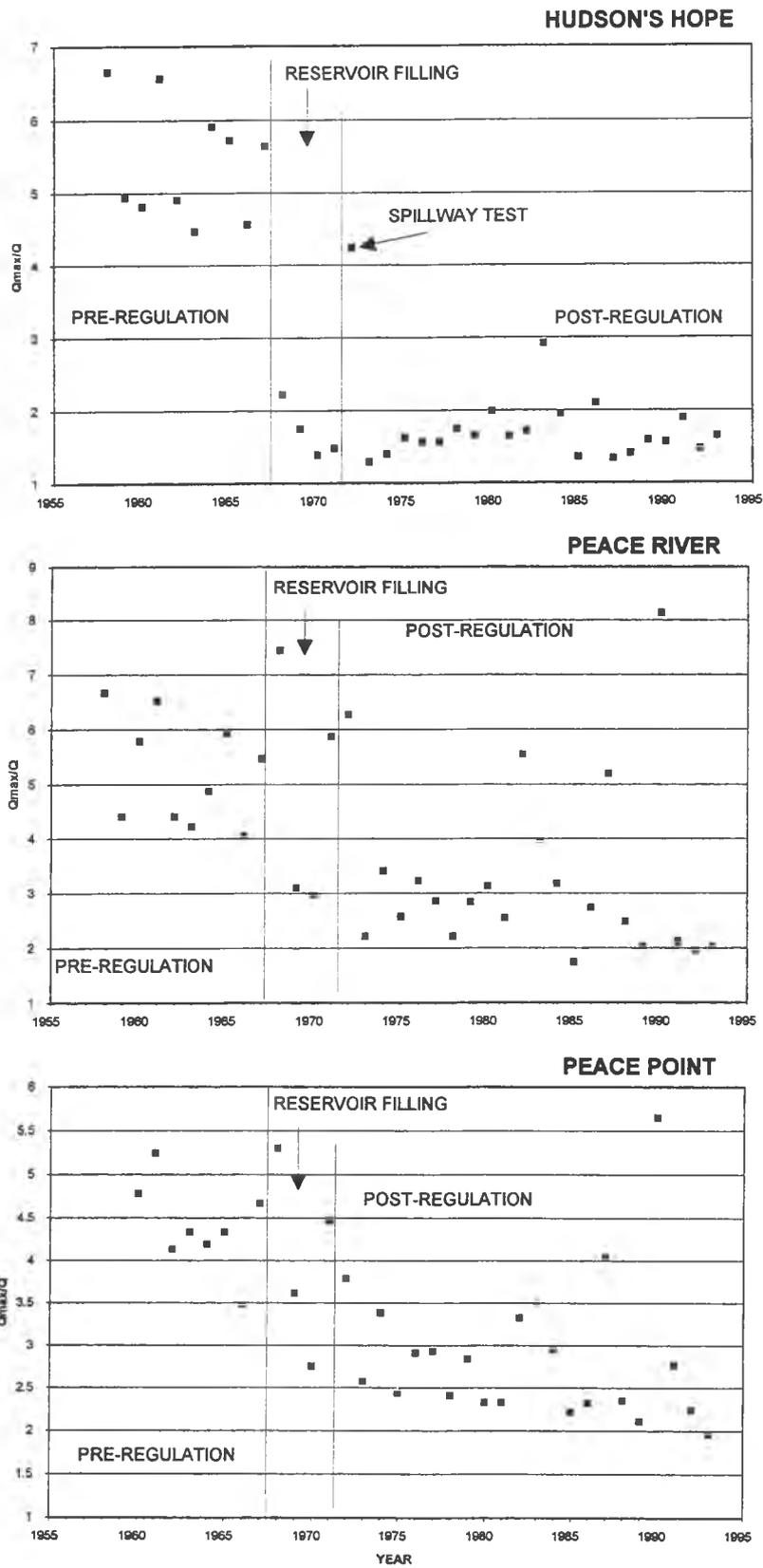
**Figure 5. Time sequences of the ratio  $Q_{max}/\langle Q \rangle$  (annual maximum daily flow/annual mean flow) at principal gauging stations along Peace River (complete duration of records).**
