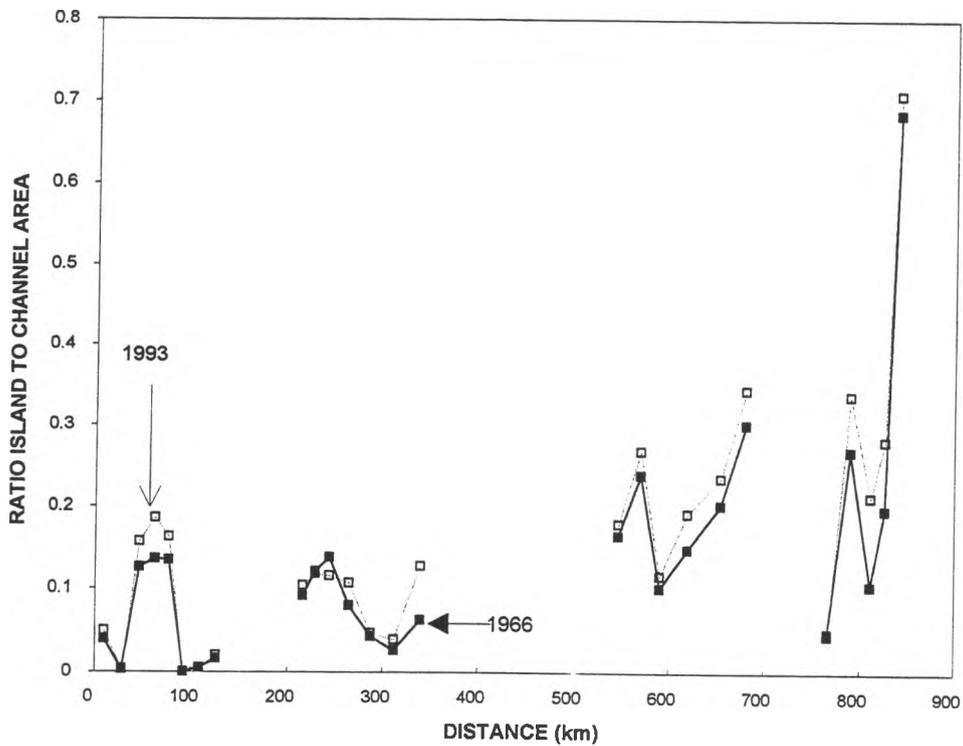
**Figure 23. (a) Downstream variation of the ratio of total bar area to channel area in Peace River for 1968 and 1993, by subreach. Distances are measured downstream from the British Columbia - Alberta border; (b) Downstream variation of the ratio of island area to channel area in Peace River for 1968 and 1993, by subreach; distances downstream from the British Columbia - Alberta border.**
