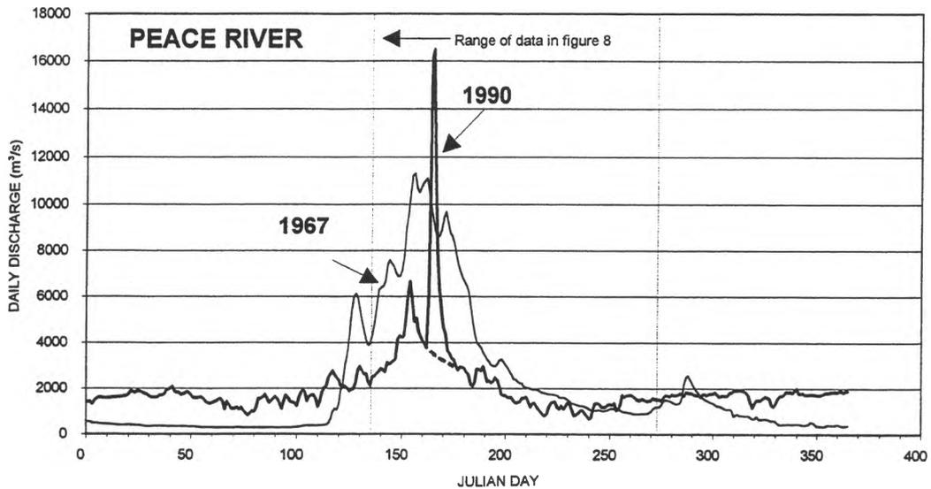
**Figure 7. Annual hydrographs at Hudson's Hope, British Columbia (immediately downstream from W.A.C.Bennett Dam) and Peace River town for 1967 (pre-regulation) and 1990. The 1990 hydrograph at Peace River includes the flood of record. The pecked line under the flood peak indicates the more usual post-regulation hydrograph.**
