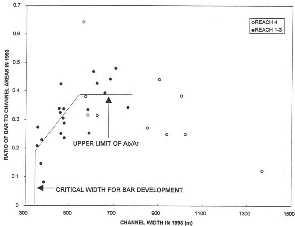
Figure 22. Ratio of total bar area (bare + vegetated) to channel zone area as a function of channel width in 1993: includes only the upstream portion of reach 4.
