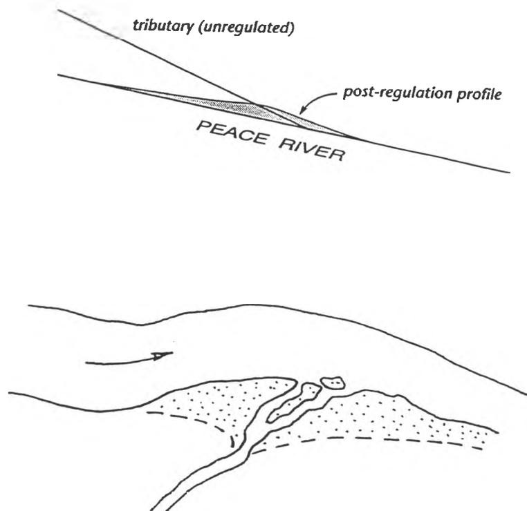
**Figure 14. Typical situation of prograding fan blocking Peace River at principal tributary confluence.**
