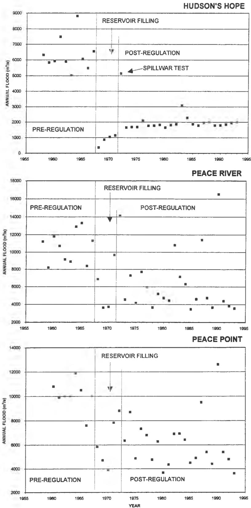
**Figure 4. Time sequences of annual maximum flow (daily at principal gauging stations along Peace River (complete duration of records)).**
