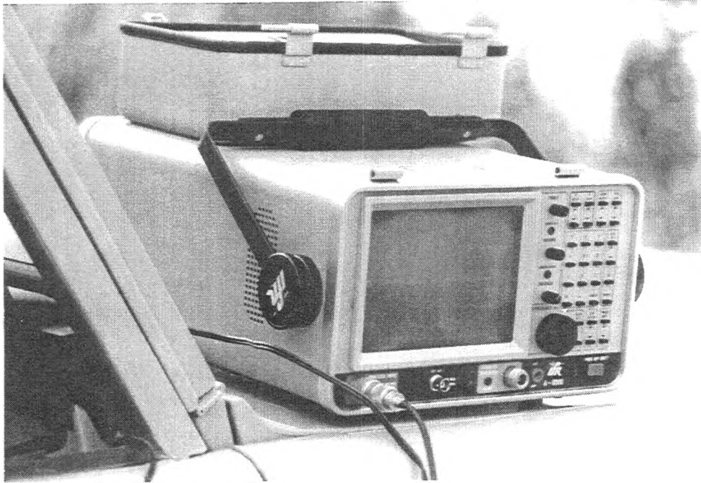
Photo #1 IFR Model 8000 portable spectrum analyzer used to conduct noise scans.
