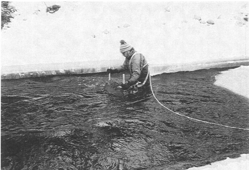
Plate 42. Through ice kick netting of invertebrates for contaminant analysis at Site 5 - Blue Ridge.
