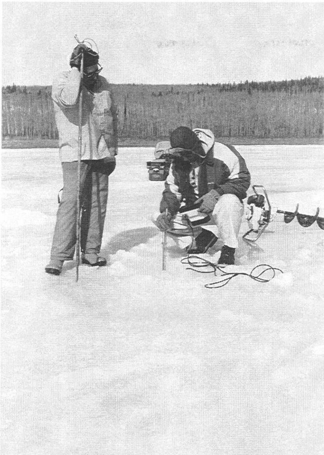
Plate 29. Checking depth and velocity with Marsh-McBirney velocity meter.
