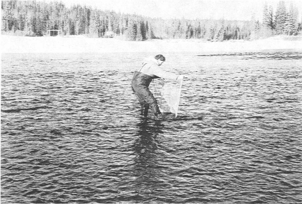
Plate 41. Open water kick netting of invertebrates for contaminant analysis at Site 2 - Weldwood Haul Bridge.
