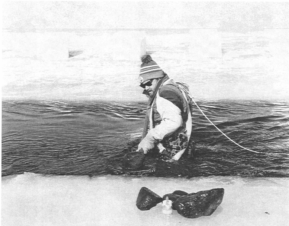
Plate 39. Lifting substrate with a steel shovel for biofilm sampling.
