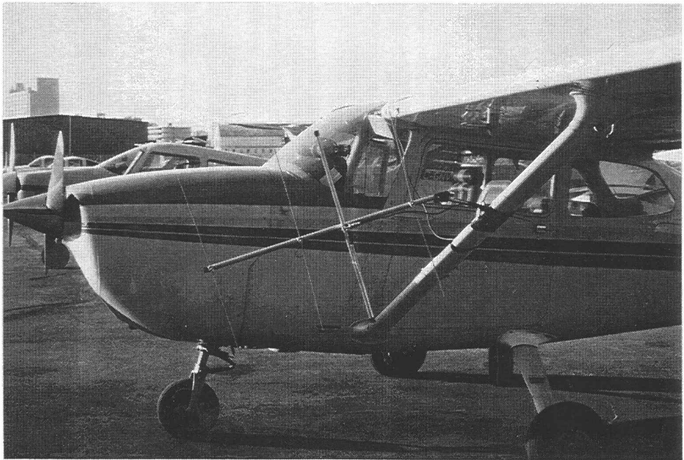
Photo #3 Yagi antenna mounted on Cessna 172.
