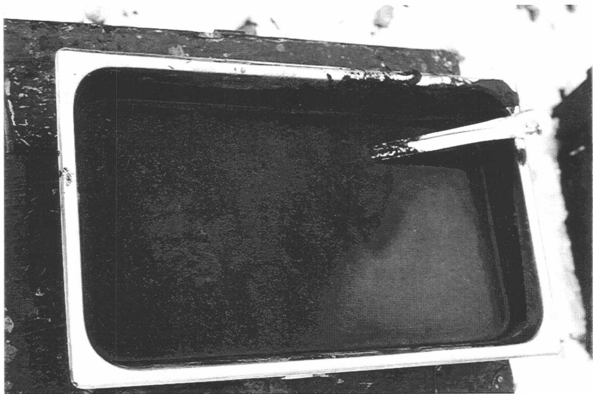
Composite of erosional sediments at Site 2 (near Weldwood Haul Bridge). Note the black organic fines.
